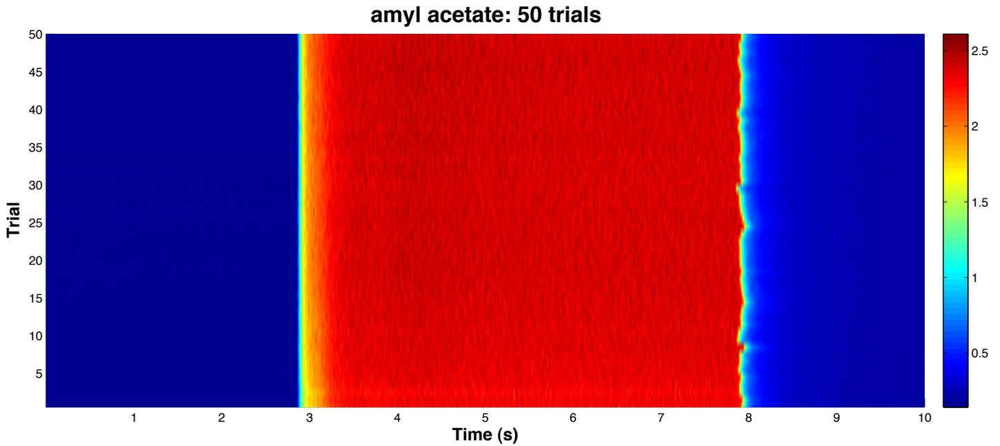
Fig. 5 - 50 repeats of the PID response to amyl acetate using the experimental setup shown in Fig. 3. One of these repeats is shown in Fig.4. Here the 50 repeats are stacked on each other to form a heat map. Each trial is represented as a horizontal bar where the color of the bar is at any given point corresponds to the amplitude of the PID response signal. The amplitude of the signal is coded according to the color key on the right.
