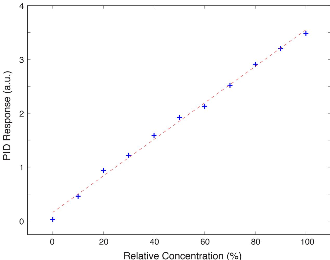
Fig.1 - Dilution measurements of amyl acetate. Dilutions were achieved by adjusting the relative flow rates of the carrier and dilution gases while keeping the total flow constant. The dashed red line is a best fit to the data.
