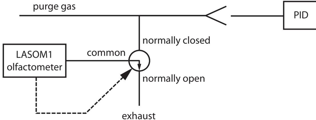
Fig. 3 - Experimental setup for repeatability and jitter measurements. The olfactometer controlled (dashed line) an external 3-way Teflon solenoid valve that was used to create an odor event with precise timing. The PID itself has a pump that is used to bring gases into the instrument.
