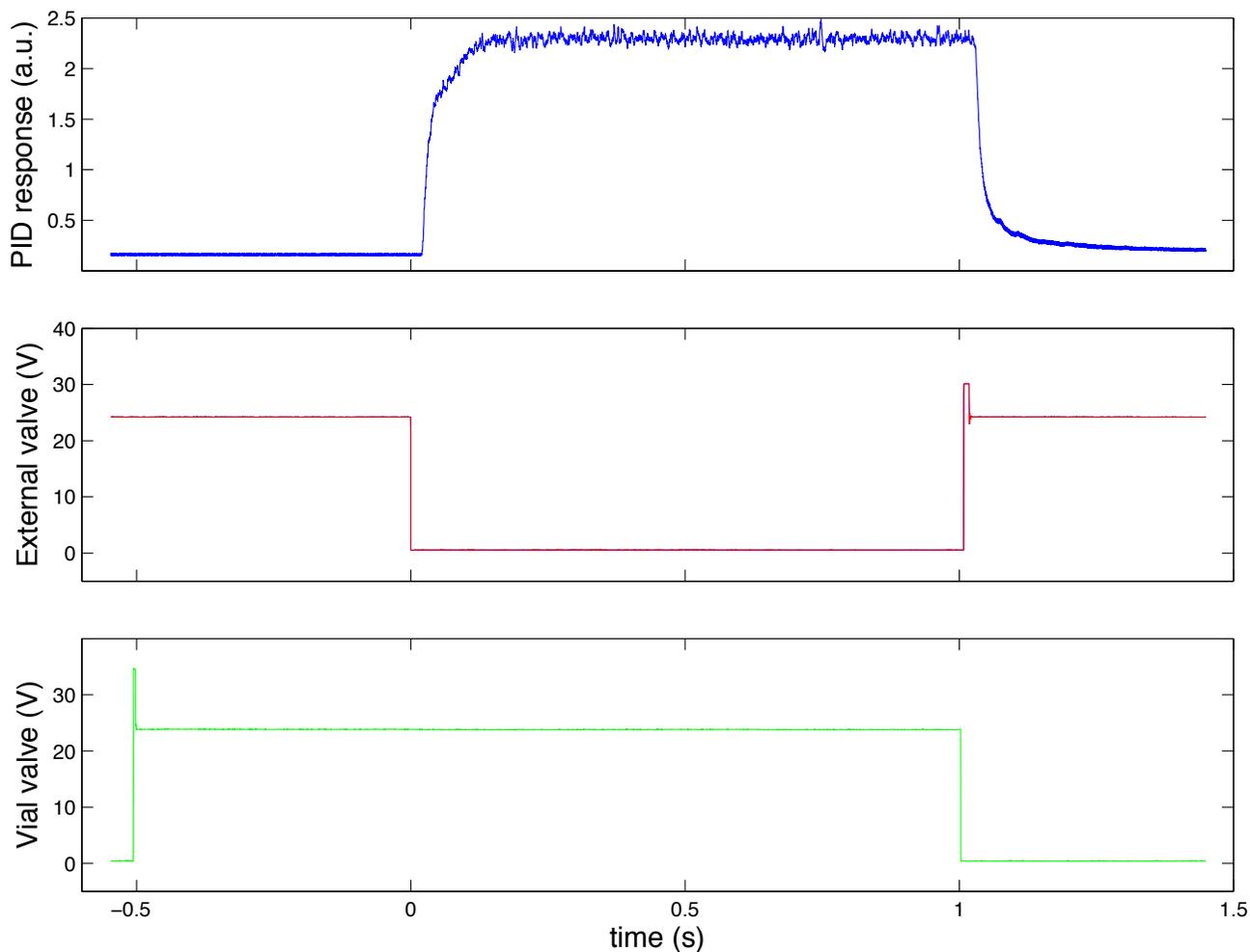
Fig. 4 - Example of the PID response (top trace) to a pulse of an amyl acetate. An external valve was used for this measurement (see Fig. 3). First, a steady state of odor output from the olfactometer is prepared. Then, the external valve is used to present the odor to the PID. This arrangement allows for more precise timing of the olfactory signal.
