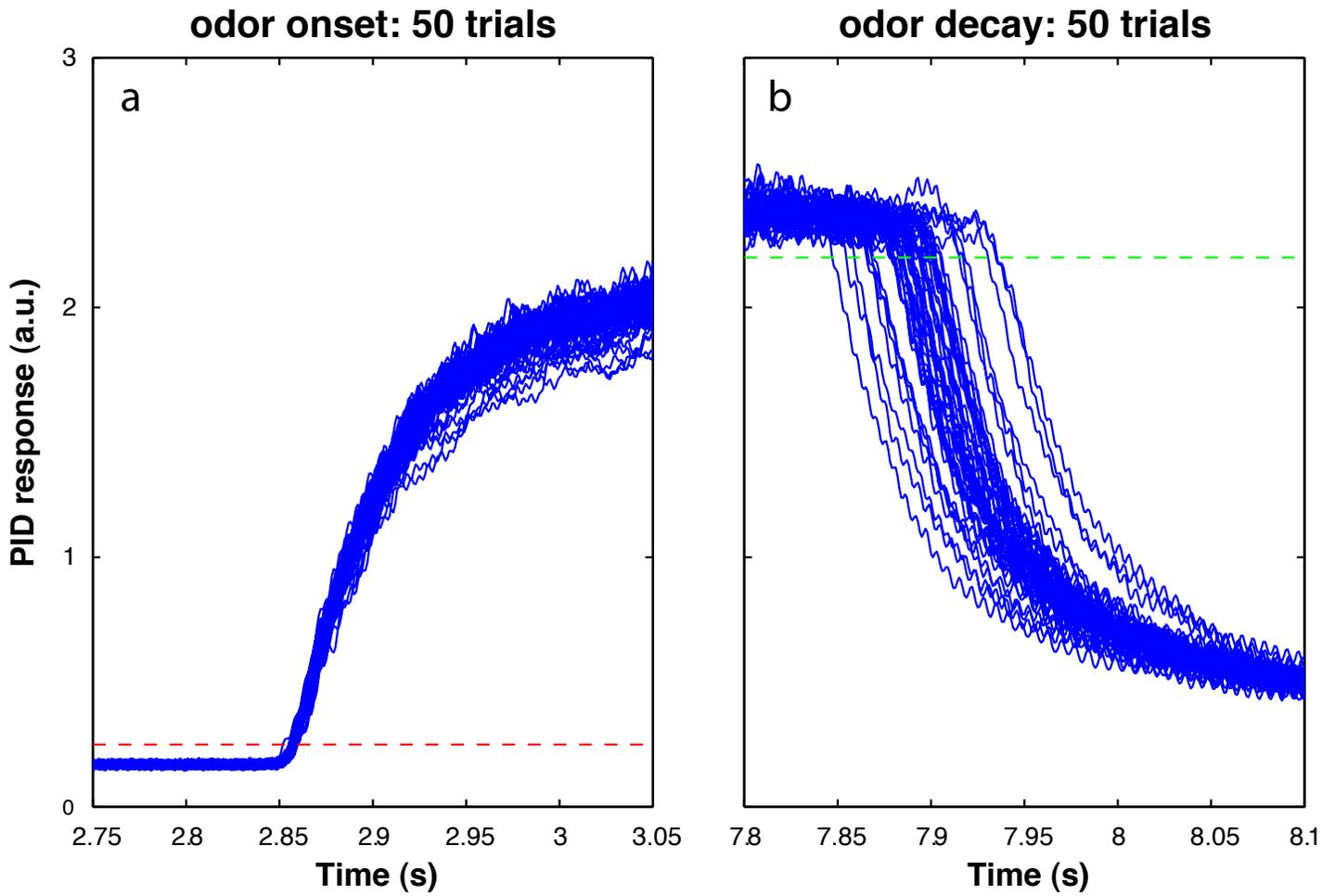
Fig. 6 - Rise and fall time of the odor signal as measured by the PID. The red and green lines are the threshold values used to calculate the jitter in the rise and fall times.
