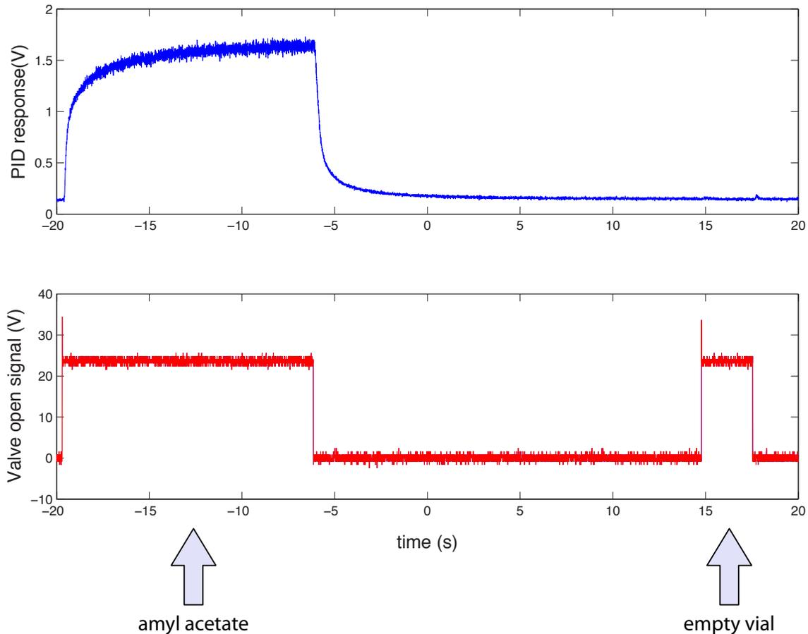
Fig. 2 - Cross contamination measurements. The PID response to the downstream clean vial contents shows that very little if any cross contamination occurs. The tiny artifact that appears when the vial 10 valve was closed was most likely induced electrical noise from the valve driver.
